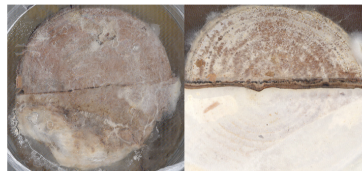
Figure 3. Wood disc inoculated with fungi and treated with heat. 100 °C for 25 min. The disc on the right is a untreated control. The upper fungi is P. gigantea (fire associated species) and the lower is F. pinicola (non fire associated species).
